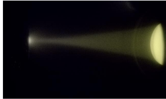
Figure 4b: Focused plasma beam of the plasma beam source (right: plasma beam source; left: substrate) with the large coupling electrode, a power of 400 W, a pressure of 2 \times 10^{-4} mbar and a magnetic coil setting of G0M0.7.
